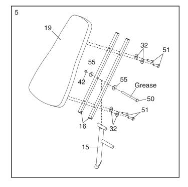
6. Apply a portion of the included grease to an M10 x 165mm Bolt (50). Attach the Backrest Frames (16) to the Frame (1) with the Bolt, two M10 Washers (55), and an M10 Nylon Locknut (42). Set the end of the Backrest Post (15) in one of the slots in the Frame. Do not overtighten the Nylon Locknut; the Backrest Frames must pivot easily.
